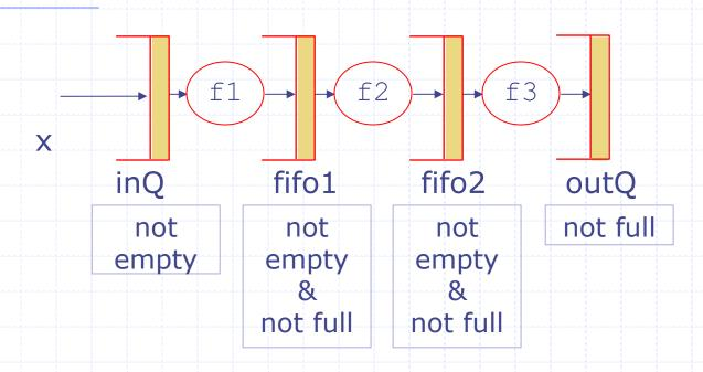
At best alternate stages in the pipeline will be able to fire concurrently
