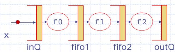
Elastic: A pipeline stage can process data if its input FIFO is not empty and output FIFO is not Full
