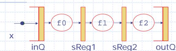
Inelastic: all pipeline stages move synchronously
