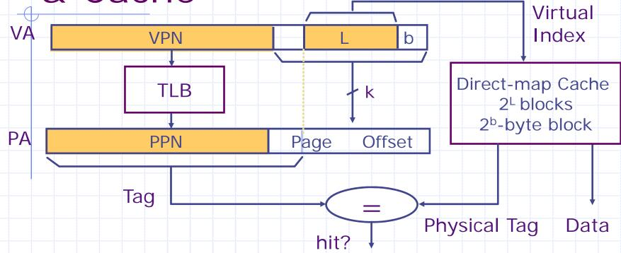
Index L is available without consulting the TLB ⇒ cache and TLB accesses can begin simultaneously Tag comparison is made after both accesses are completed
