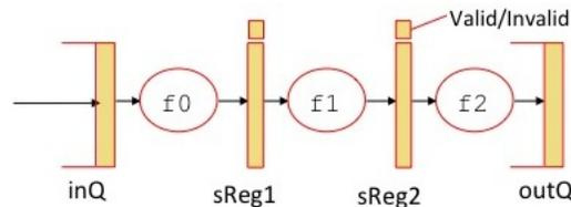
Figure 4.4: Valid bits on pipeline registers
