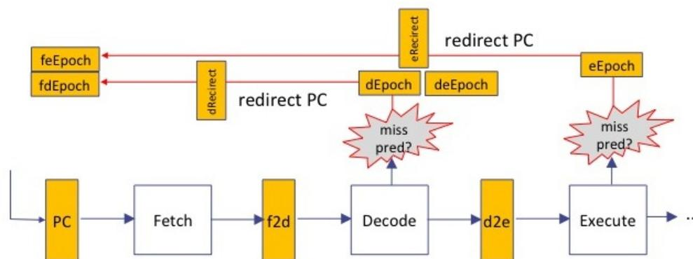
Figure 10.11: N-stage pipeline, with two predictors
