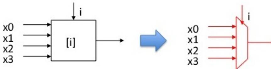
Figure 2.4: Bit-select circuit, dynamic index
