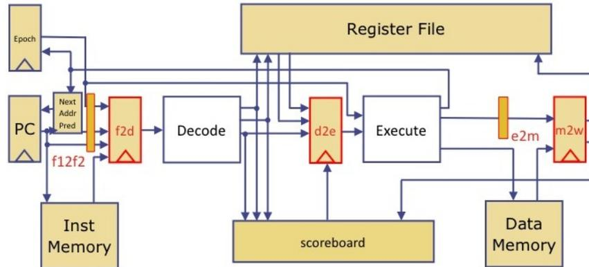
Figure 12.10: Integrating caches into the pipeline
