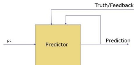
Figure 10.3: Dynamic prediction is a feedback control system
