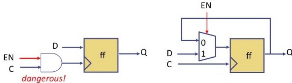
Figure 3.3: Implementing a D flip-flop with Write-Enable
