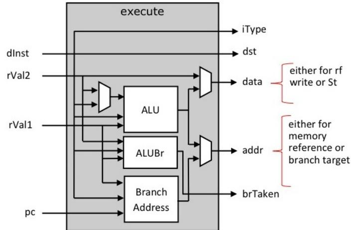
Figure 5.8: SMIPS processor Execute function
