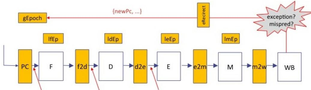
Figure 11.4: Redirection logic in the processor pipeline
