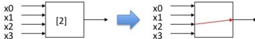
Figure 2.3: Bit-select circuit, static index
