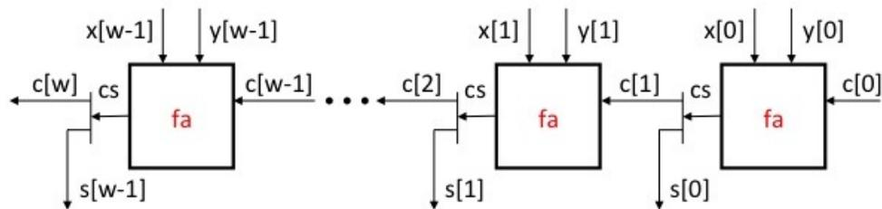
Figure 2.5:  $w$ -bit Ripple Carry Adder circuit
