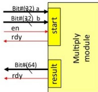
Figure 7.2: Hardware interpretation of interface methods
