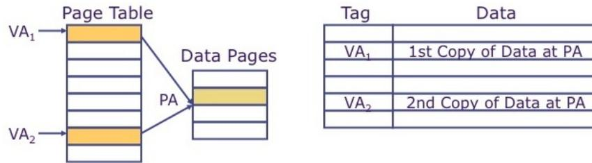
Figure 13.18: Aliasing in virtually-addressed caches
