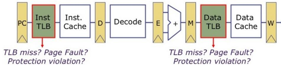
Figure 13.16: Virtual Memory operations in the processor pipeline
