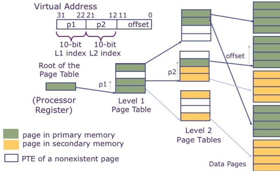
Figure 13.7: Hierarchical page tables for large, sparse address spaces
