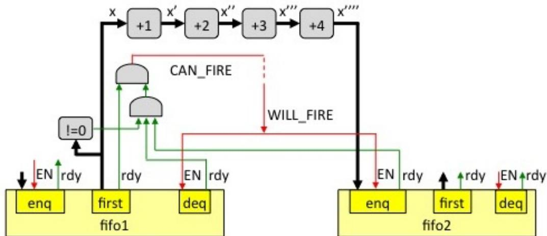
Figure 7.6: Combinational circuit for a rule: another example
