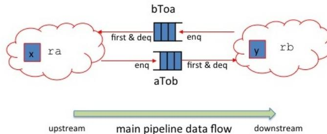
Figure 8.2: Typical Pipeline and Bypass FIFO usage
