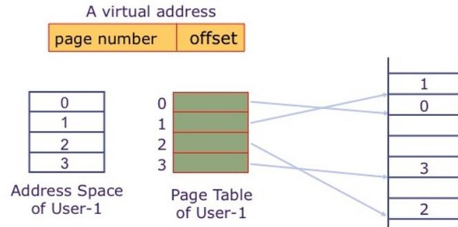
Figure 13.3: Mapping VAs to PAs using a page table
