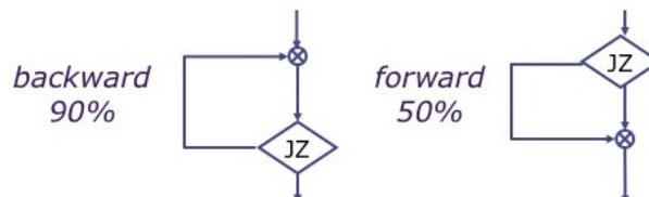
Figure 10.2: Branch probabilities for forward and backward branches
