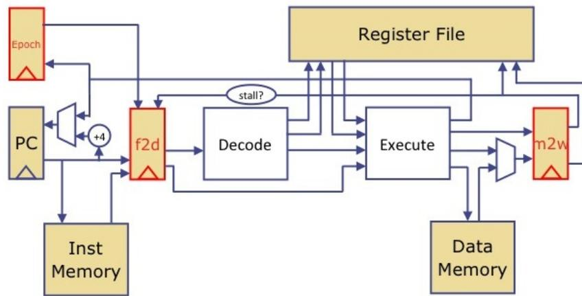
Figure 12.1: 4 stage pipeline
