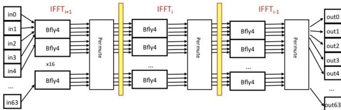
Figure 4.2: Pipelined Inverse Fast Fourier Transform (IFFT)
