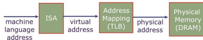
Figure 13.2: Various kinds of addresses in a Virtual Memory system
