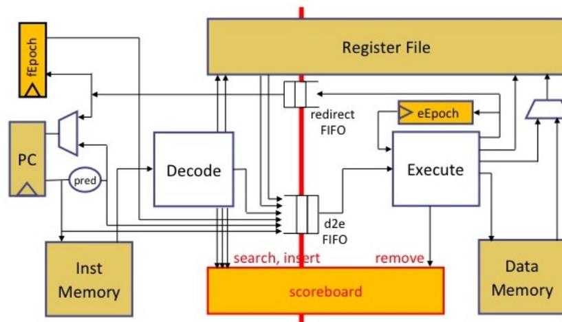
Figure 9.4: Pipeline with scoreboard
