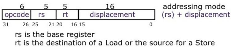
Figure 5.3: SMIPS processor Computational and Load/Store instruction formats
