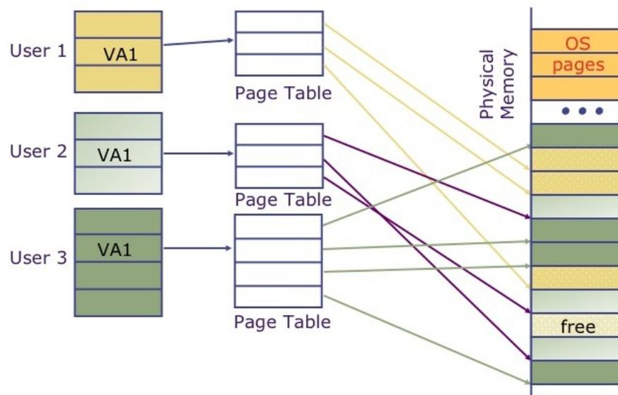
Figure 13.4: Multiple address spaces using multiple page tables
