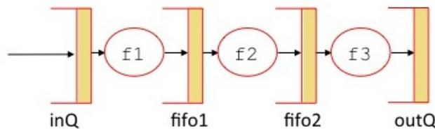
Figure 4.6: An elastic pipeline
