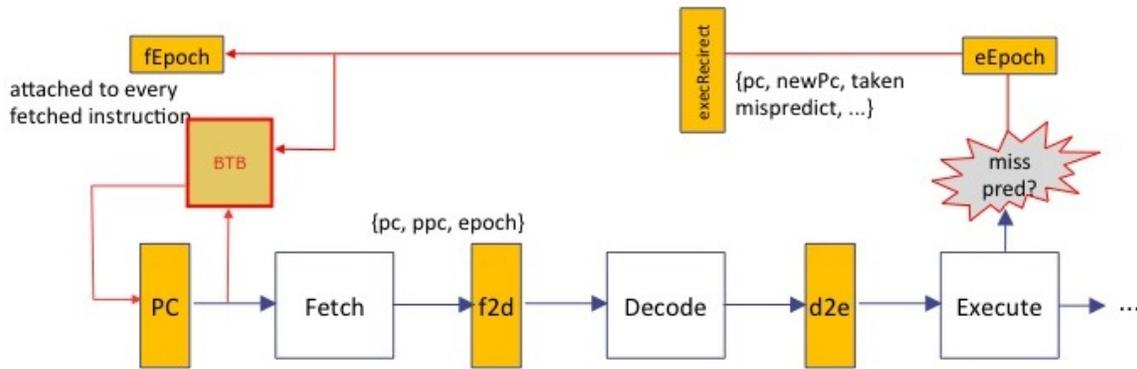
Figure 10.10: N-stage pipeline, with one predictor (BTB) only
