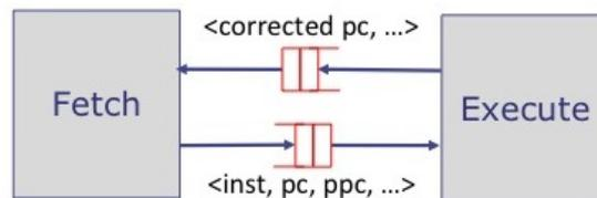
Figure 6.2: Decoupled structure
