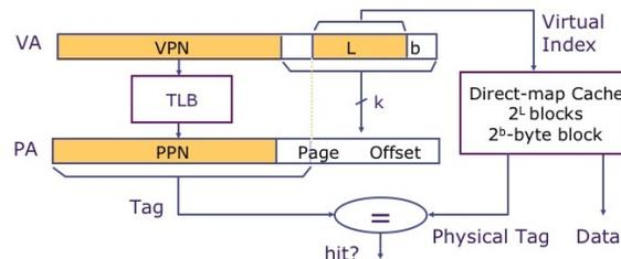
Figure 13.19: Concurrent access to the TLB and cache
