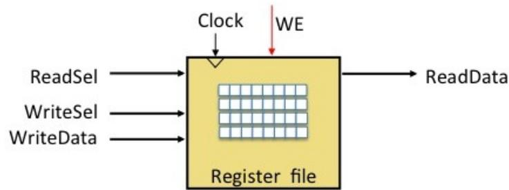
Figure 3.9: A Register File with four 8-bit registers
