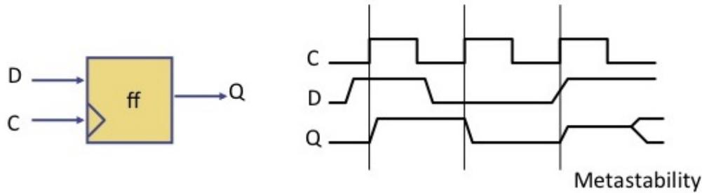
Figure 3.1: An edge-triggered D flip-flop and an example input-output waveform
