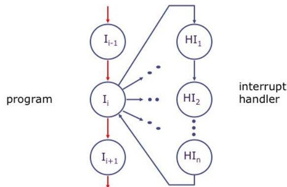
Figure 11.1: Instruction flow on an interrupt
