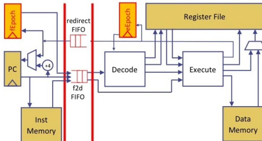
Figure 6.5: Decoupled solution
