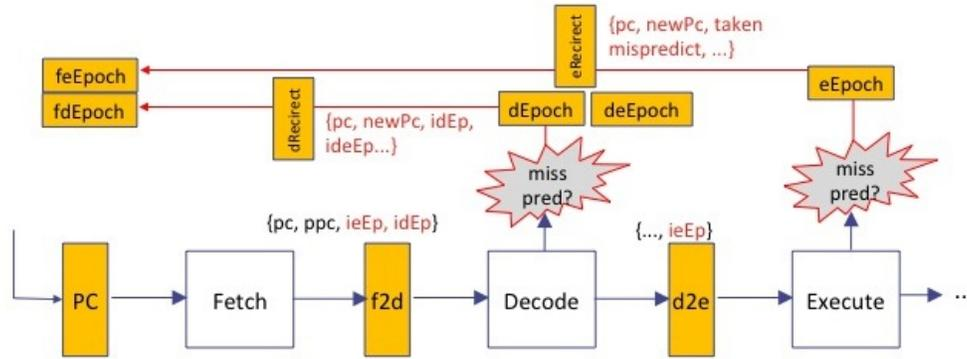
Figure 10.12: N-stage pipeline, with two predictors and redirection logic
