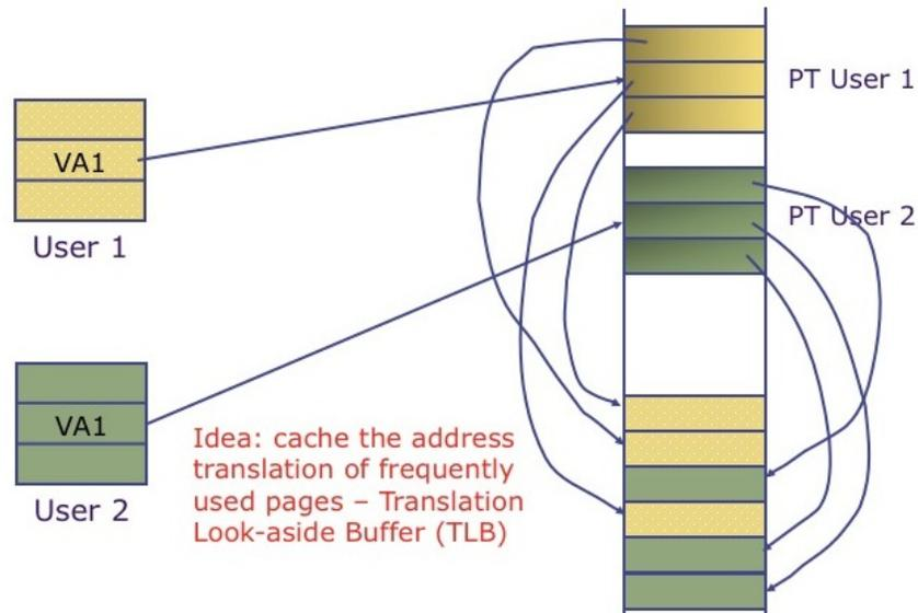
Figure 13.6: Page table for multiple address spaces in physical memory
