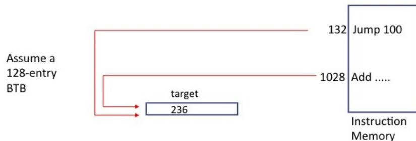
Figure 10.6: Address collisions in the simple BTB
