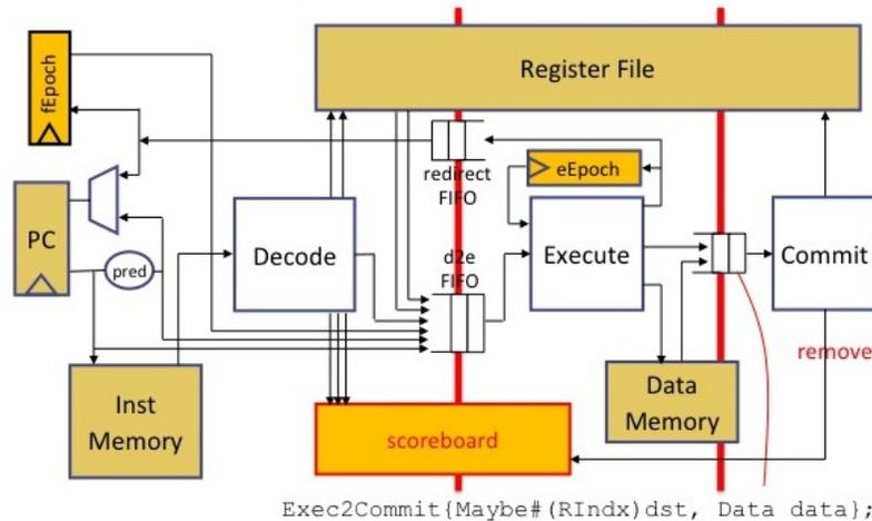
Figure 9.6: 3-stage pipeline
