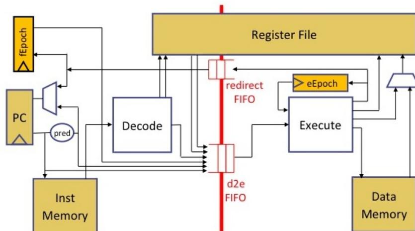
Figure 9.1: Alternate two-stage pipelining of SMIPS
