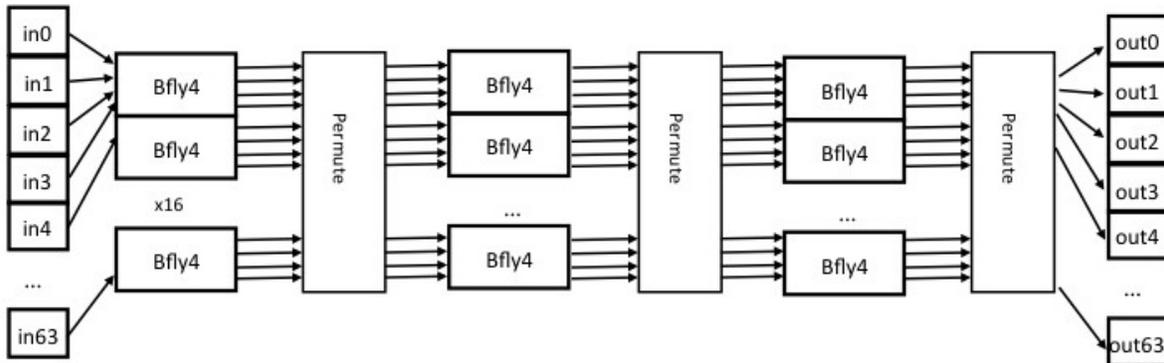
Figure 4.1: Combinational Inverse Fast Fourier Transform (IFFT)
