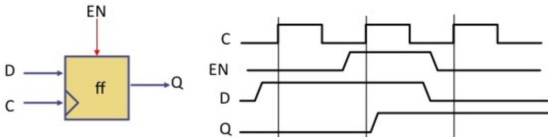
Figure 3.2: A D flip-flop with Write-Enable
