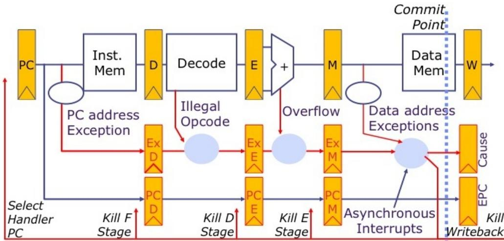
Figure 11.3: Exception handling in the processor pipeline
