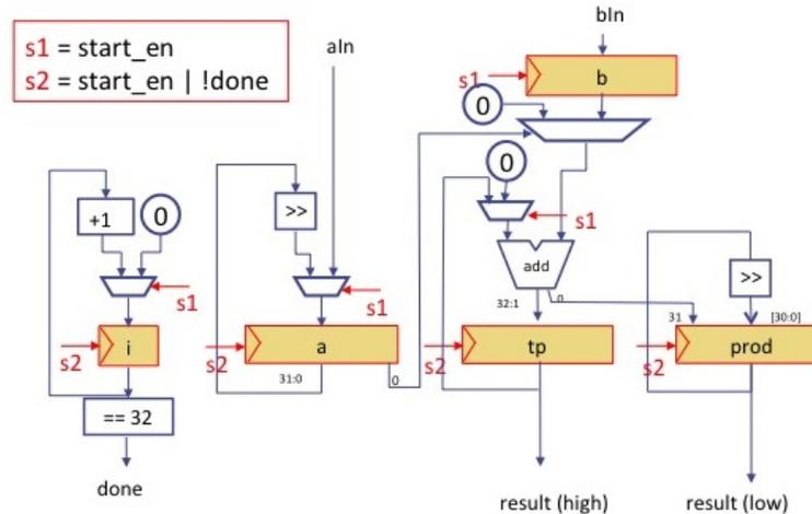
Figure 3.6: Sequential multiplication circuit
