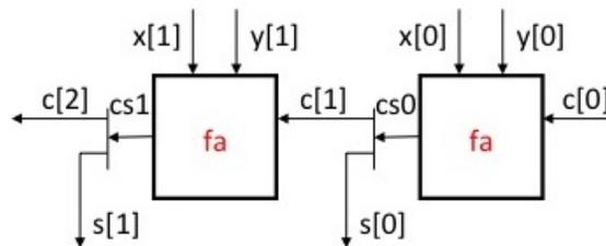
Figure 2.2: 2-bit Ripple Carry Adder circuit
