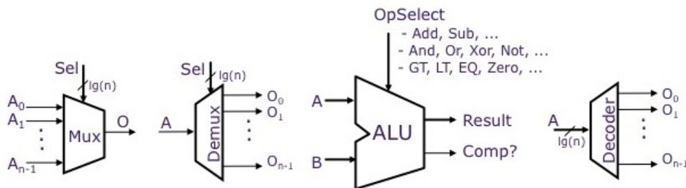
Figure 2.13: Various combinational circuits
