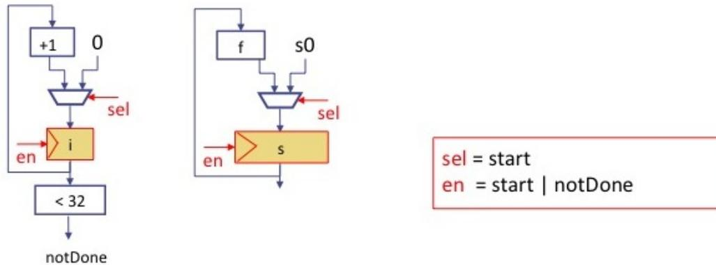
Figure 3.5: Circuit implementation of C iteration example
