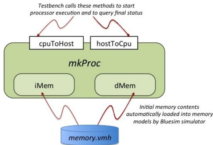
Figure 5.5: Uniform interface for running our implementations
