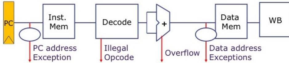
Figure 11.2: Synchronous interrupts raised at various points in the pipeline
