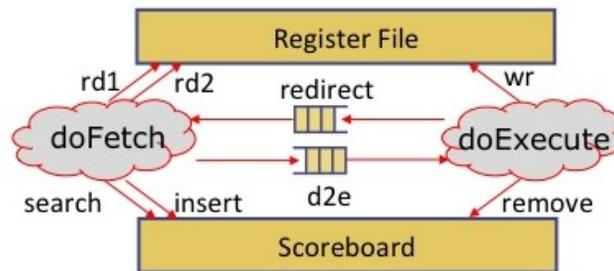
Figure 9.5: Abstraction of the pipeline for concurrency analysis
