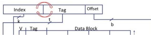
Figure 12.6: Choice of which bits to use in a direct mapped cache
