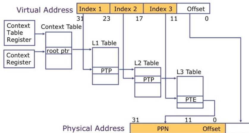
Figure 13.12: Hierarchical Page Table Walk in SPARC v8
