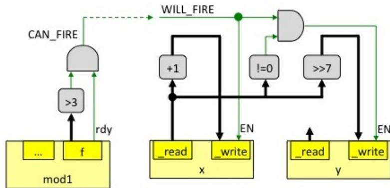
Figure 7.5: Combinational circuit for a rule
