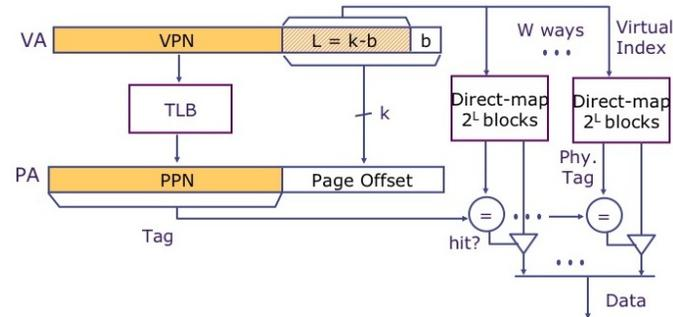
Figure 13.20: A cache with virtual index and physical tag
