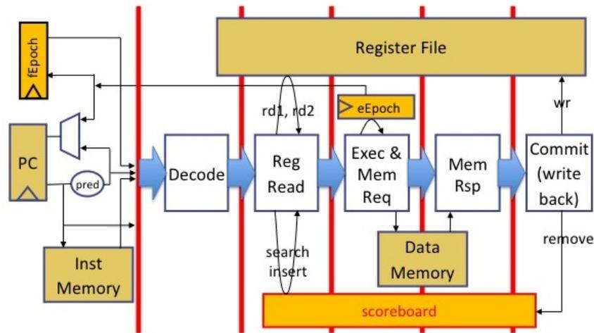
Figure 9.7: 6-stage pipeline
