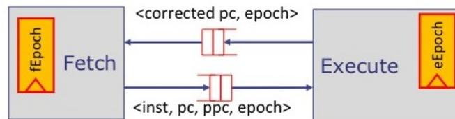
Figure 6.3: Adding epoch registers to distributed units
