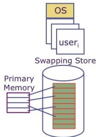
Figure 13.1: Virtual Memory by Paging between physical memory and secondary store
