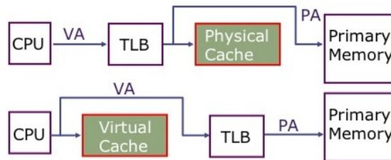
Figure 13.17: Caches based on Virtual or Physical Addresses
