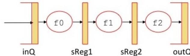
Figure 4.3: Inelastic pipeline for IFFT
