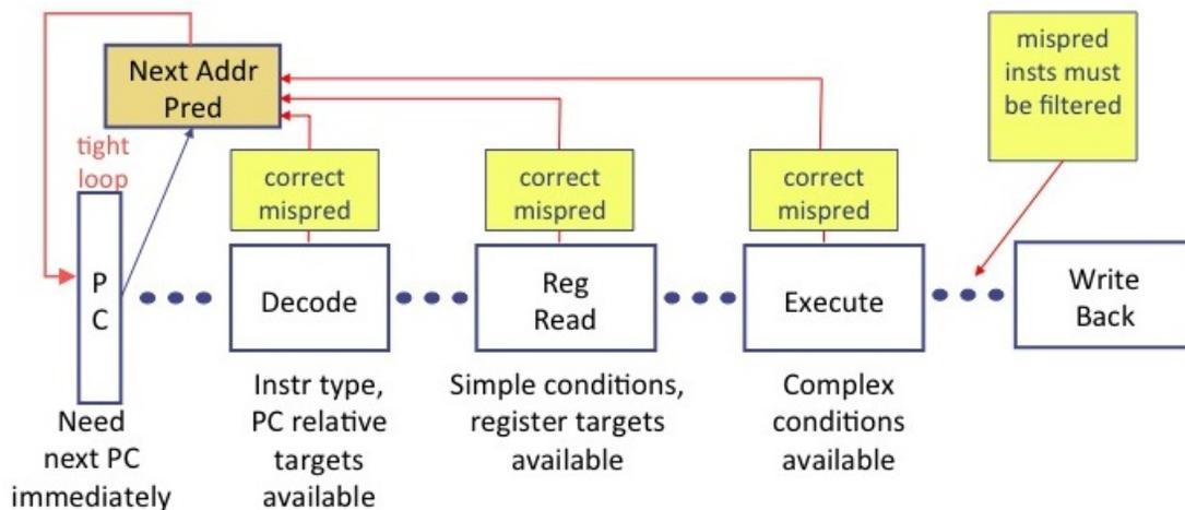
Figure 10.4: Overview of control flow prediction
