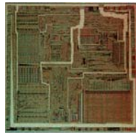
Intel 8086, 1978, 33mm 2 10Mhz, 29K transistors, 3u
