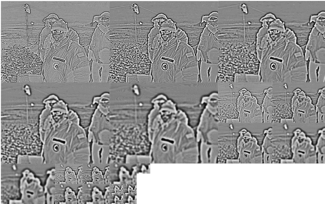
Figure 6: All DoG levels generated by hardware; contrast has been increased.
