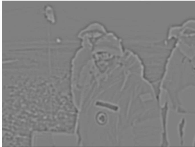
Figure 5: Difference between two Gaussians generated by hardware.
