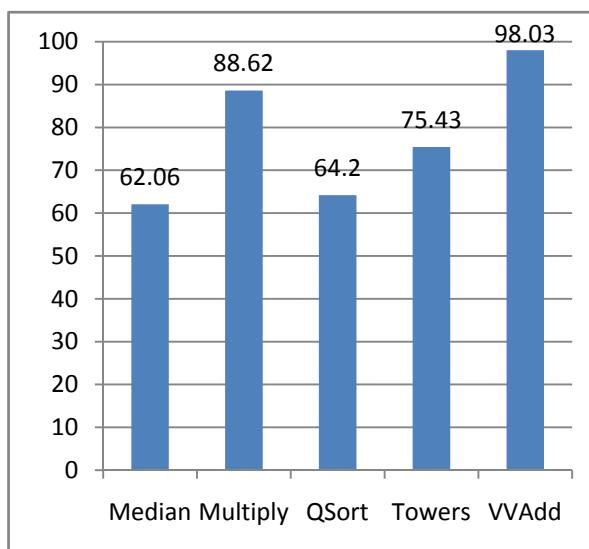
Figure 4-3 1-bit Branch Predictor Accuracy
