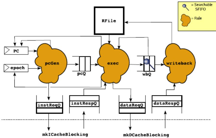
Figure 3-1 Lab5 SMIPS Processor
