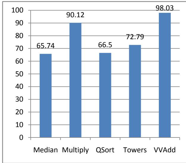
**Figure 4-6 2-bit Branch Predictor Accuracy**
