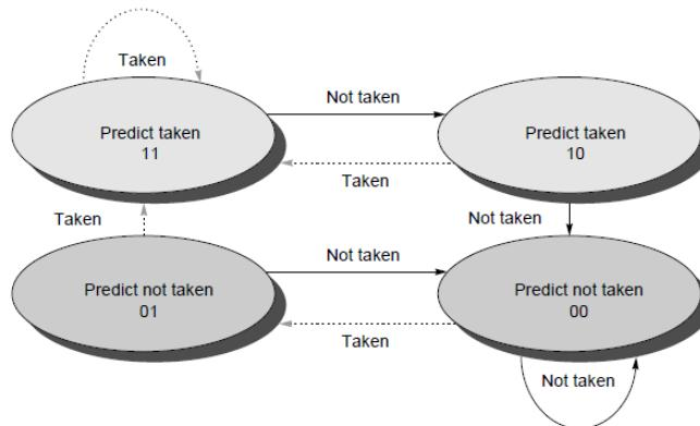
Figure 4-5 2-bit Branch Predictor State Transition Diagram
