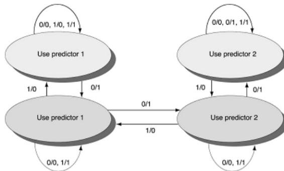
**Figure 4-7 Tournament 2-bit Branch Predictor State Transition Diagram**
