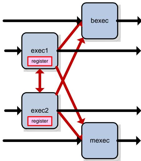
**Figure 4-10 Intra-Module Result Sharing Architecture**
