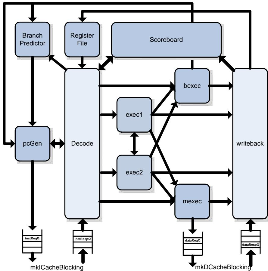
Figure 4-1 Superscalar Processor Implementation
