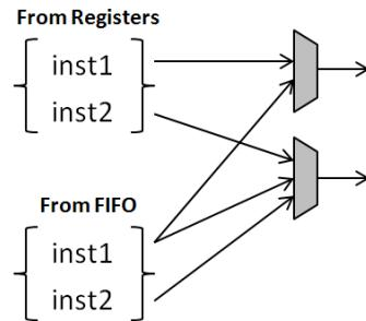
Figure 4-9 Conceptual Representation of Decode Permutation Stage
