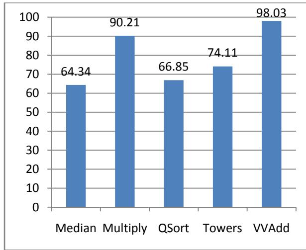
Figure 4-8 Tournament 2-bit Branch Predictor Accuracy
