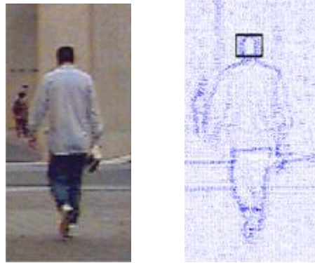
Figure 2: A typical pedestrian training image (left) and its gradient (right)
