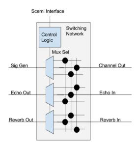
The switching matrix is comprised of a series of multiplexers that redirect the output of each block to the next block. These multiplexers are controlled by a control logic unit that decodes the block order from a Sce-Mi interface and routes the signals accordingly. The calculated selection bits are stored in registers until the system is reconfigured.
