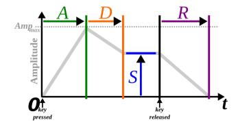
The signal quickly rises to a peak amplitude during the attach phase before dropping to an amplitude that is held for the duration of the note. When the note is released, it slowly decays back to zero. Almost any instrument can be mimicked by making the attack, decay, and release times, in addition to the sustain level, programmable.
