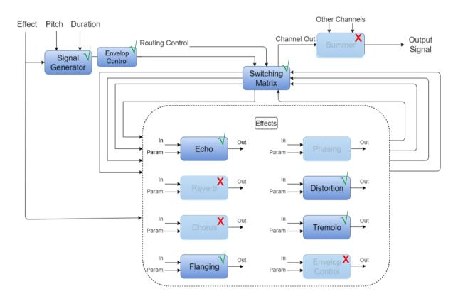
The diagram above depicts the high-level diagram of the implemented system. The Signal Generator, Switching Matrix and Envelop Control blocks were considered the most critical ones. The Effects showed were initial ideas before the implementation. The final design had four of them: Echo, Flanging, Distortion, and Tremolo. The location of the Envelope generator was moved to simplify architecture design.
