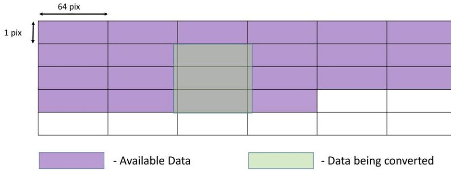
Figure 10. Frozen State of Modified Sobel Module. Helpful for cycle analysis.
