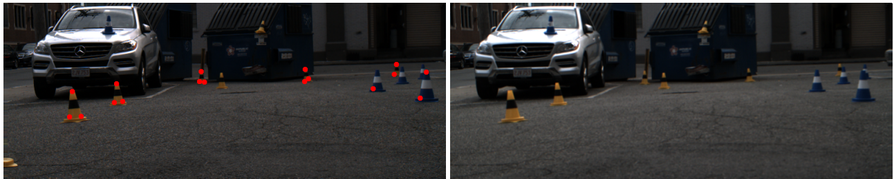
Figure 1: Sample stereo images taken by the MIT Driverless Racecar. The red points on the left image represent the coordinates of the points for which we want to compute real-world position coordinates using the stereo vision algorithm.
