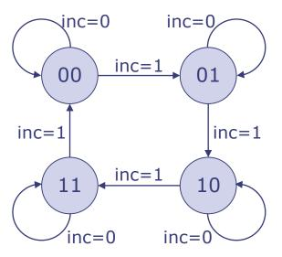
Finite State Machine (FSM) representation
