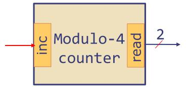
interface Counter; method Action inc; method Bit#(2) read; endinterface
