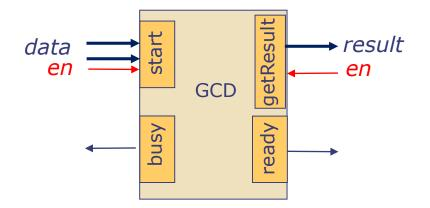
GCD can be started if the module is not *busy*; Results can be read when *ready*
