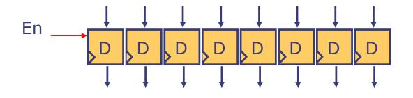
*Register:* A group of flip-flops with a common clock and enable
