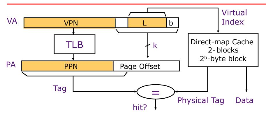
Index L is available without consulting the TLB ⇒ cache and TLB accesses can begin simultaneously Tag comparison is made after both accesses are completed
