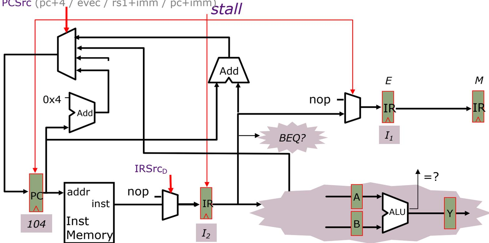
Branch condition is not known until the execute stage. *What action should be taken in the decode stage?*
