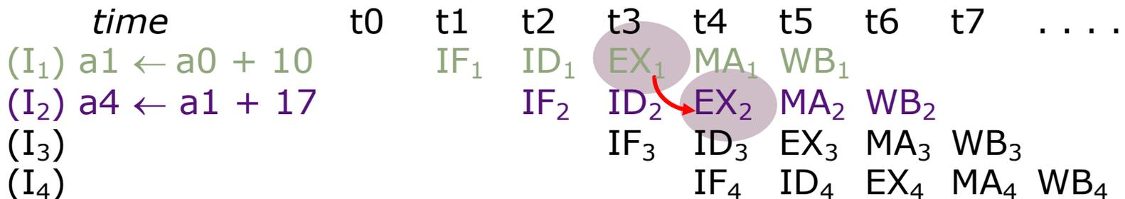
A new datapath, i.e., a *bypass*, can get the data from the output of the ALU to its input
