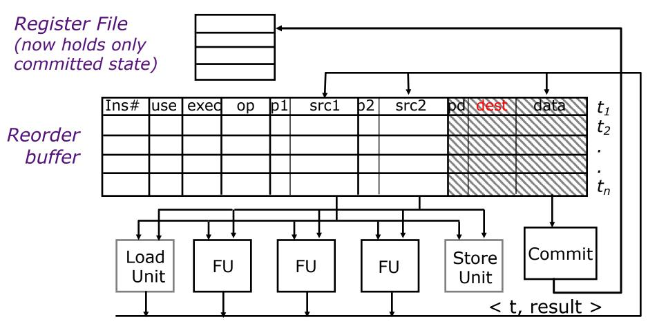
Register file does not contain renaming tags any more. How does the decode stage find the tag of a source register?
