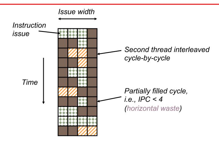
What is the effect of cycle-by-cycle interleaving?
