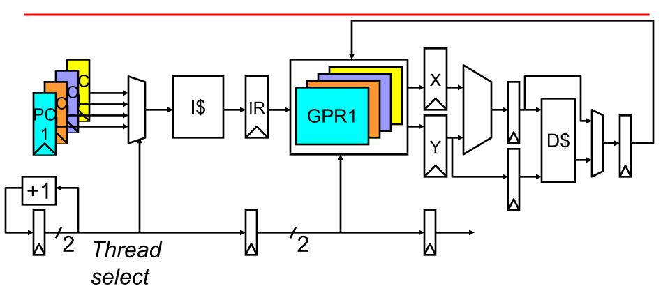
Have to carry thread select down pipeline to ensure correct state bits read/written at each pipe stage
