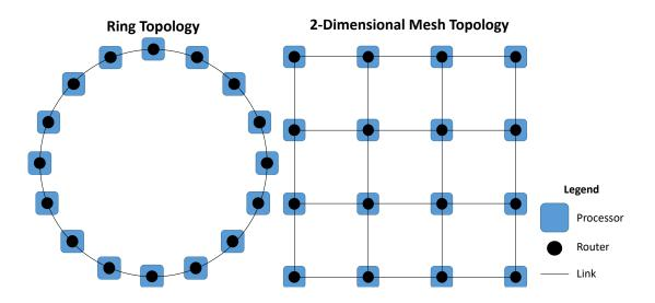
Assuming that there are N nodes, calculate the following for each topology. Assume uniform random traffic for average distance calculation. For the average distance of the mesh, you can answer in terms of its asymptotic growth with respect to N (e.g.,  $O(N^3)$ ).
