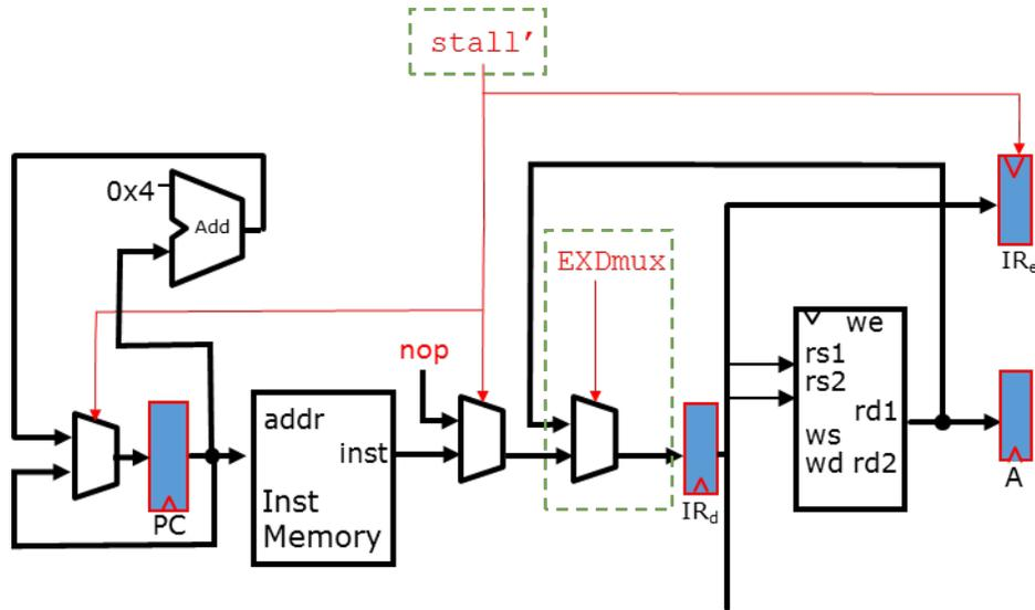
Your task is to write the new stall signal (`stall'`) and fill in the missing signal, `EXDmux`. Write your signal in terms of signals (e.g., `PC` or `rd1` or `IRD`) and feel free to use the old stall signal (`stall`).
