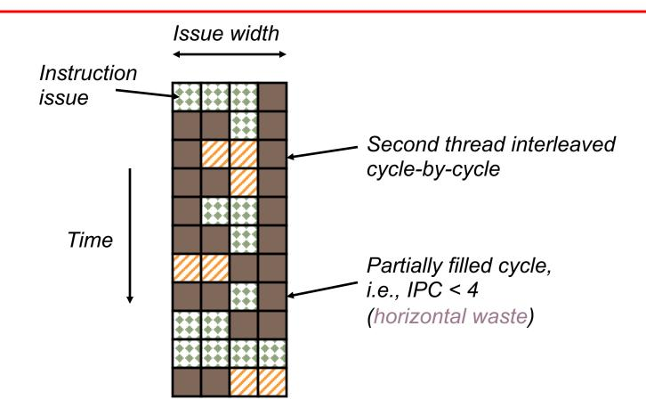
What is the effect of cycle-by-cycle interleaving?
