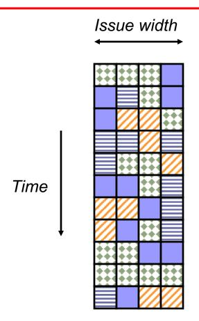
Interleave multiple threads to multiple issue slots with no restrictions
