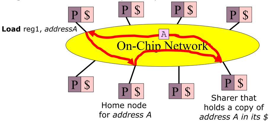
Network transports cache coherence messages and cache lines between processor cores
