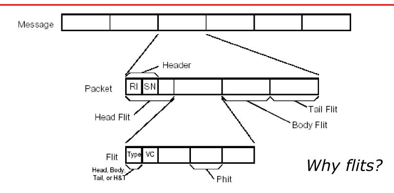
Packet: Basic unit of routing and sequencing
