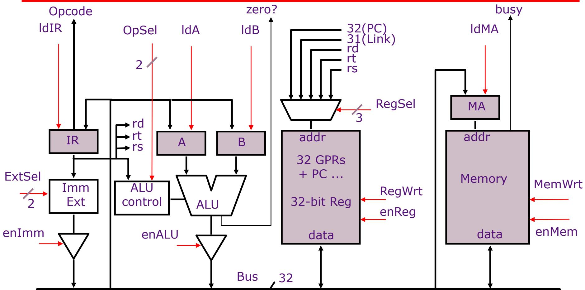
*Microinstruction: register to register transfer (17 control signals)*
