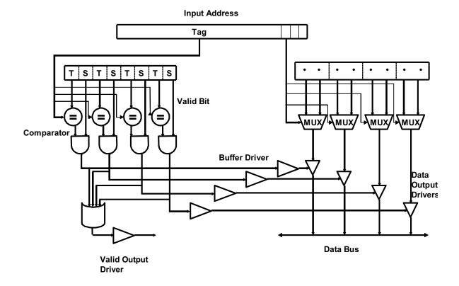
Please complete Table M3.2-1 below with delays across each element of the cache. Using the data you compute in Table M3.2-1, calculate the critical path delay through this cache (from when the Input Address is set to when both Valid Output Driver and the appropriate Data Output Driver are outputting valid data).
