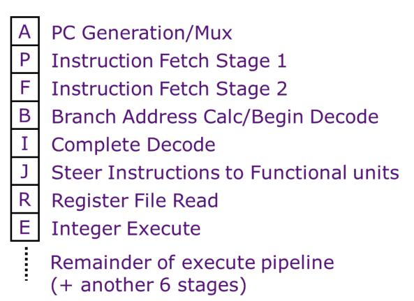
You are designing a processor with the complex pipeline illustrated above. For this problem assume there are no unconditional jumps or jump register—*only* conditional branches.
