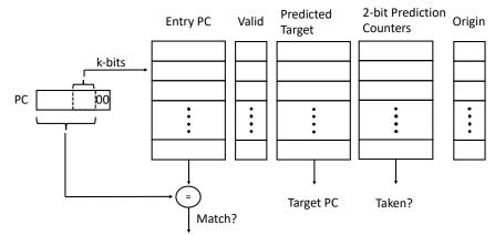
A BTB hit indicates one of the two instructions in the instruction bundle is predicted as a taken branch, and the processor fetches the next instruction bundle from the target PC. A BTB miss indicates that no branch is found within the instruction bundle, and the processor simply fetches the next sequential instruction bundle.
