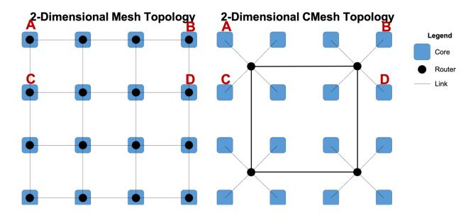
Instead of assigning a single core per router, the cmesh topology allows four cores to share one router. Thus, there is a factor of 4 reduction in the number of routers needed.
