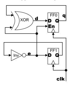
Fill out the state transition diagram for the sequential logic drawn above.
