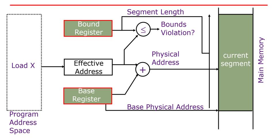
Base and bounds registers are visible/accessible only when processor is running in the *supervisor mode*
