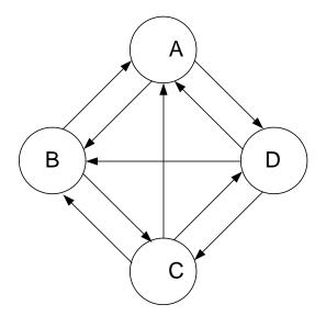
Note that each link is unidirectional, and only one link exists between A and C (only a link from C to A (not from A to C), and only from D to B between B and D. Each link can transfer 1 flit per cycle and there is only one virtual channel per link. For all parts, 180-degree turns are not allowed.
