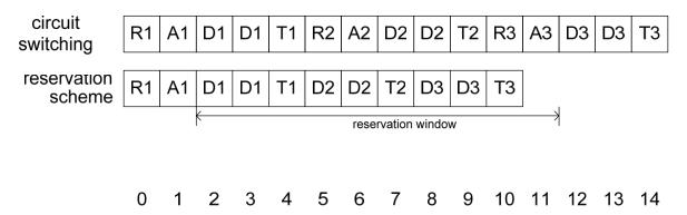
Note that tail flits may be able to get eliminated in this new scheme if they are used only to indicate when channels can be deallocated.
