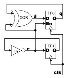
Fill out the state transition diagram for the sequential logic drawn above.
