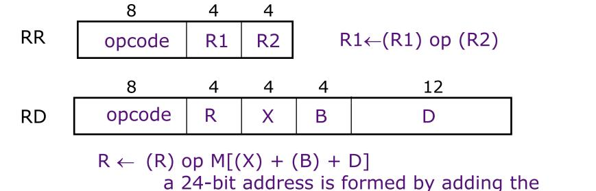
12-bit displacement (D) to a base register (B) and an Index register (X), if desired
