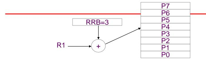
Rotating Register Base (RRB) register points to base of current register set. Value added on to logical register specifier to give physical register number. Usually, split into rotating and non-rotating registers.
