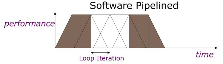
Software pipelining pays startup/wind-down costs only once per loop, not once per iteration
