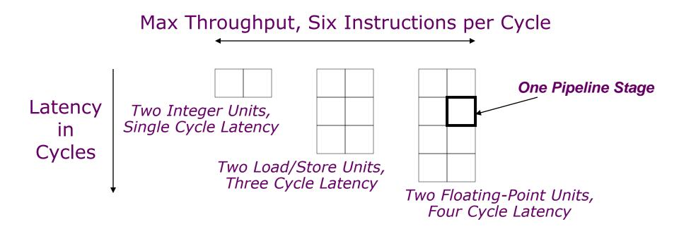
How much instruction-level parallelism (ILP) required to keep machine pipelines busy?
