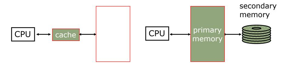
Caching cache entry cache block (~32 bytes) cache miss rate (1% to 20%) cache hit (~1 cycle) cache miss (~100 cycles) a miss is handled in hardware
