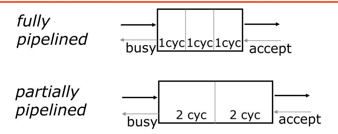
Functional units have internal pipeline registers
