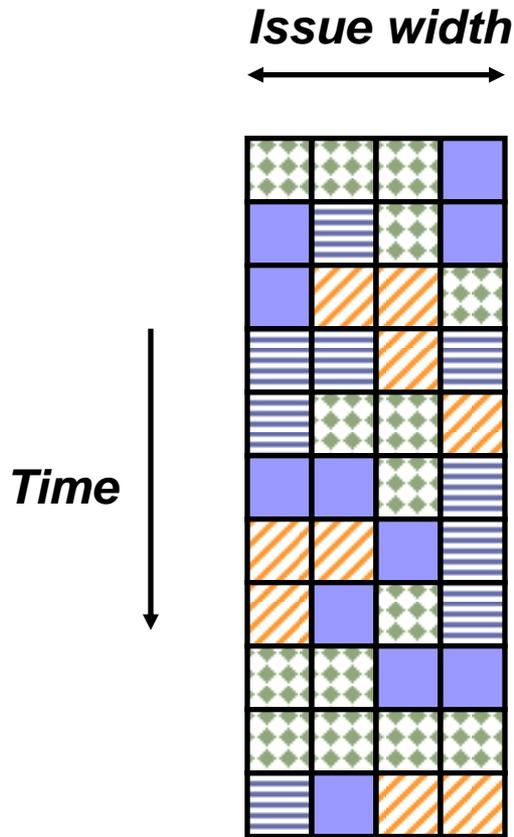
For regions with low thread level parallelism (TLP) entire machine width is available for instruction level parallelism (ILP)
