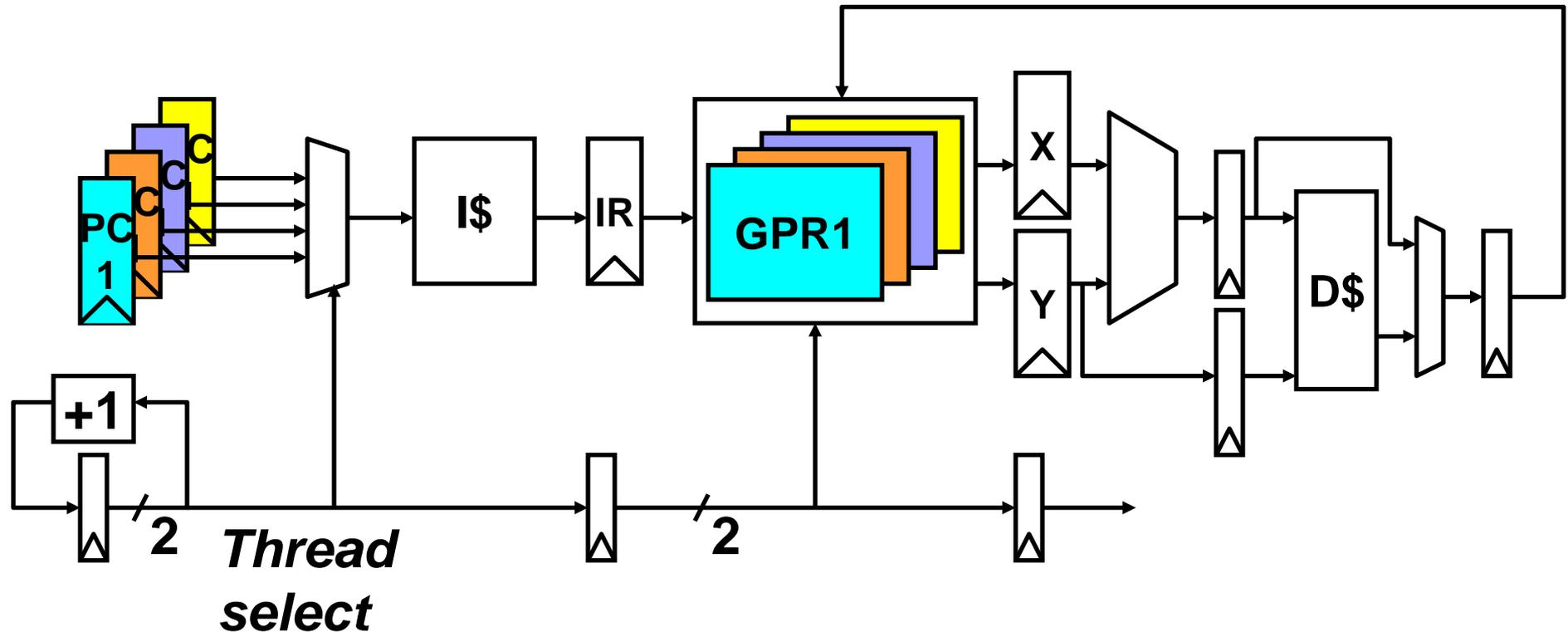
Have to carry thread select down pipeline to ensure correct state bits read/written at each pipe stage
