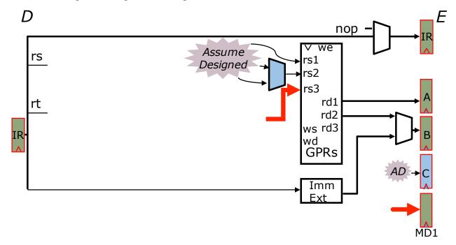
In the figure above, draw the completed datapath for a store. Assume the signals from Question 2 are already designed correctly to form a 64-bit effective address. Connect sources to the inputs of *rs3* and *MD1* (the two thick red arrows). You are free to add combinational logic as necessary.
