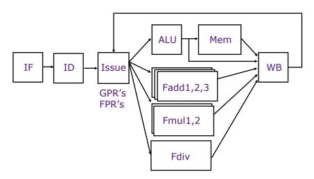
Figure H8-A: In-order MIPS Pipeline with Floating-Point Units
