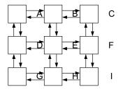
In the CDG corresponding to the mesh network above, for example,  $EF \rightarrow FC \rightarrow CB \rightarrow BE \rightarrow EF$  generates a cycle (Flow E-F-C, flow F-C-B, flow C-B-E, and flow B-E-F will generate a deadlock).
