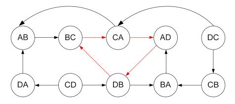
However, there are still cycles in this CDG. For example, if flow 1 from B to D is routed through B-C-A-D, flow 2 from C to B is routed through C-A-D-B, and flow 3 from A to C is routed through A-D-B-C, there can be deadlock by these three flows.
