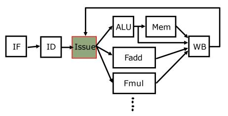
Decode does register renaming, providing a new spot for each register write
