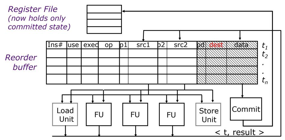
Register file does not contain renaming tags any more. How does the decode stage find the tag of a source register? Search the "dest" field in the reorder buffer
