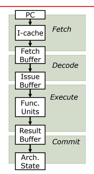
Modern processors may have > 10 pipeline stages between next PC calculation and branch resolution!
