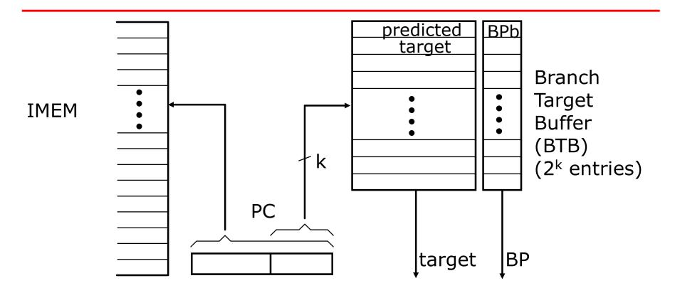
BP bits are stored with the predicted target address.
