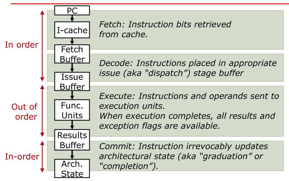
Modern processors may have > 10 pipeline stages between next PC calculation and branch resolution!
