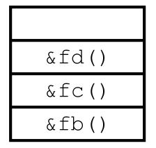
Small structure to accelerate JR for subroutine returns, typically much more accurate than BTBs.
