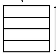
Small structure to accelerate JR for subroutine returns, typically much more accurate than BTBs.
