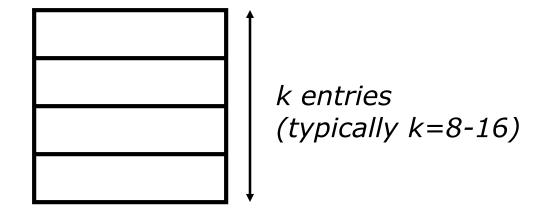
Small structure to accelerate JR for subroutine returns, typically much more accurate than BTBs.
