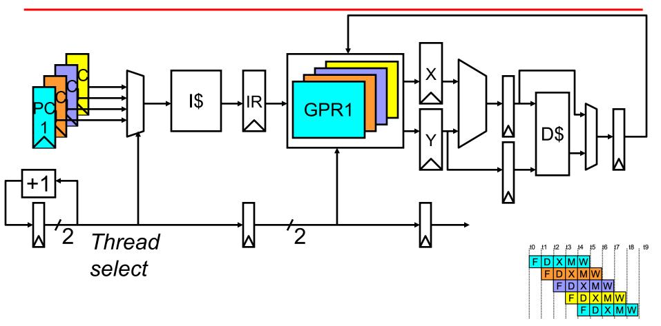
Have to carry thread select down pipeline to ensure correct state bits read/written at each pipe stage
