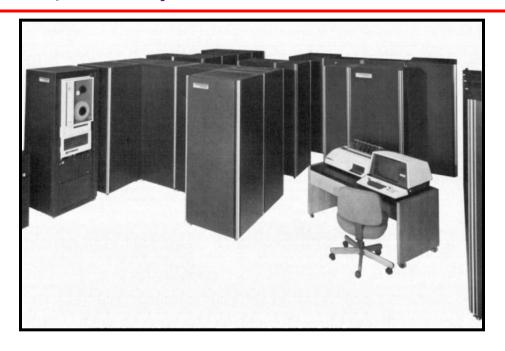
First commercial machine to use hardware threading in main CPU
