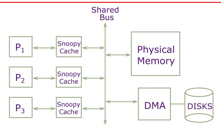
Caches watch (snoop on) bus to keep all processors' view of memory coherent
