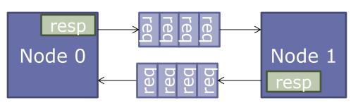
Example: Both nodes saturate all intermediate buffers with requests to each other, blocking responses from entering the network
