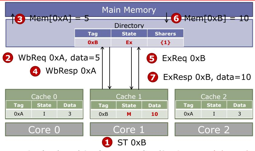
Why are 0xA's wb and 0xB's req serialized? Structural dependence Possible solutions? Buffer outside of cache to hold write data
