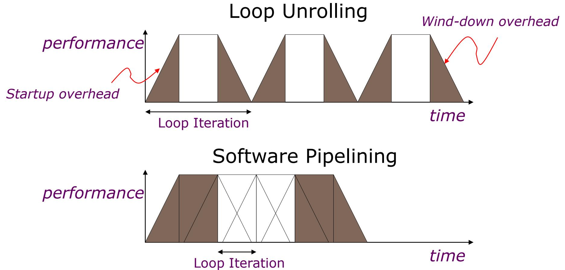
*Software pipelining pays startup/wind-down costs only once per loop, not once per iteration*
