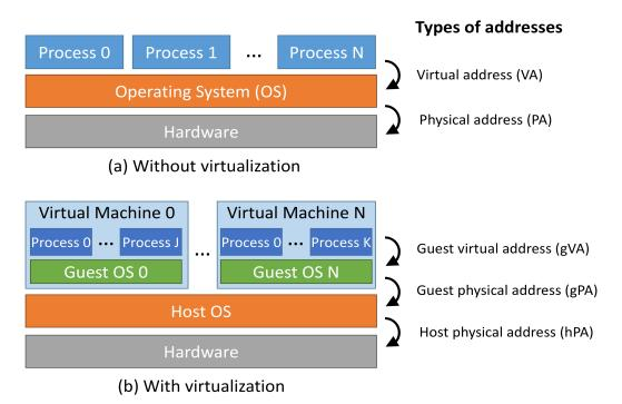
Figure 1: Key elements in systems (a) without and (b) with platform virtualization, and corresponding layers of address translation.
