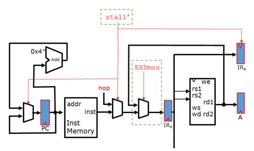
Your task is to write the new stall signal (stall') and fill in the missing signal, EXDmux. Write your signal in terms of signals (e.g., PC or rdl or IRD) and feel free to use the old stall signal (stall).
