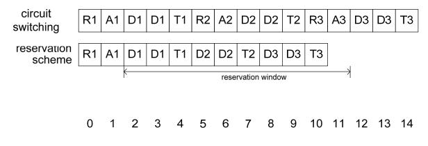
Note that tail flits may be able to get eliminated in this new scheme if they are used only to indicate when channels can be deallocated.
