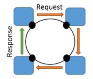
The ring with N cores has an aggregate throughput of N messages per cycle. (It is a unidirectional ring.)
