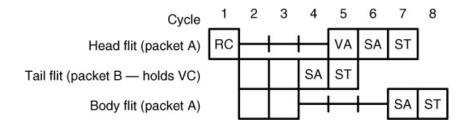
Before cycle 1, packet B's head flit has finished RC and VA. In the following cycles, packet B's four flits traverse SA and ST without stalls. Packet A's head flit completes routing computation at cycle 1 and tries to allocate an output virtual channel starting at cycle 2. Unfortunately, the only output virtual channel compatible with its route is occupied by packet B, so packet A's head flit fails to allocate a VC and is unable to make progress until packet B's tail flit releases the VC.
