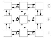
In the CDG corresponding to the mesh network above, for example,  $EF \rightarrow FC \rightarrow CB \rightarrow BE \rightarrow EF$  generates a cycle (Flow E-F-C, flow F-C-B, flow C-B-E, and flow B-E-F will generate a deadlock).
